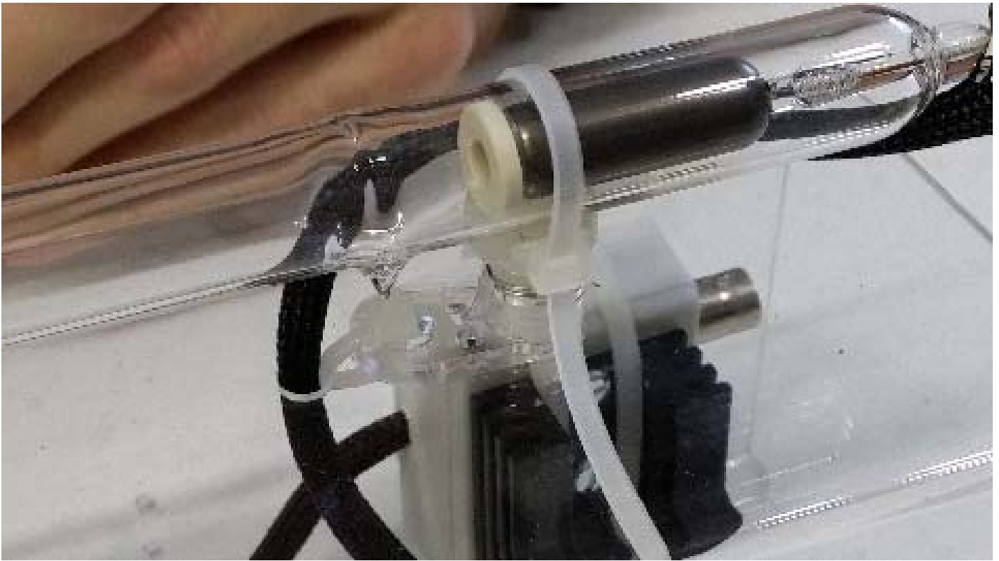
Position and Center tube on assembly. Snug up the incorporated Tie-Wrap to firmly hold tube in place
