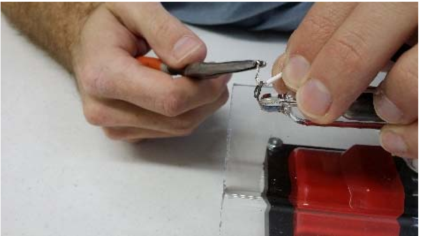
Firmly but delicately attach wires to tube electrodes on end of tube
