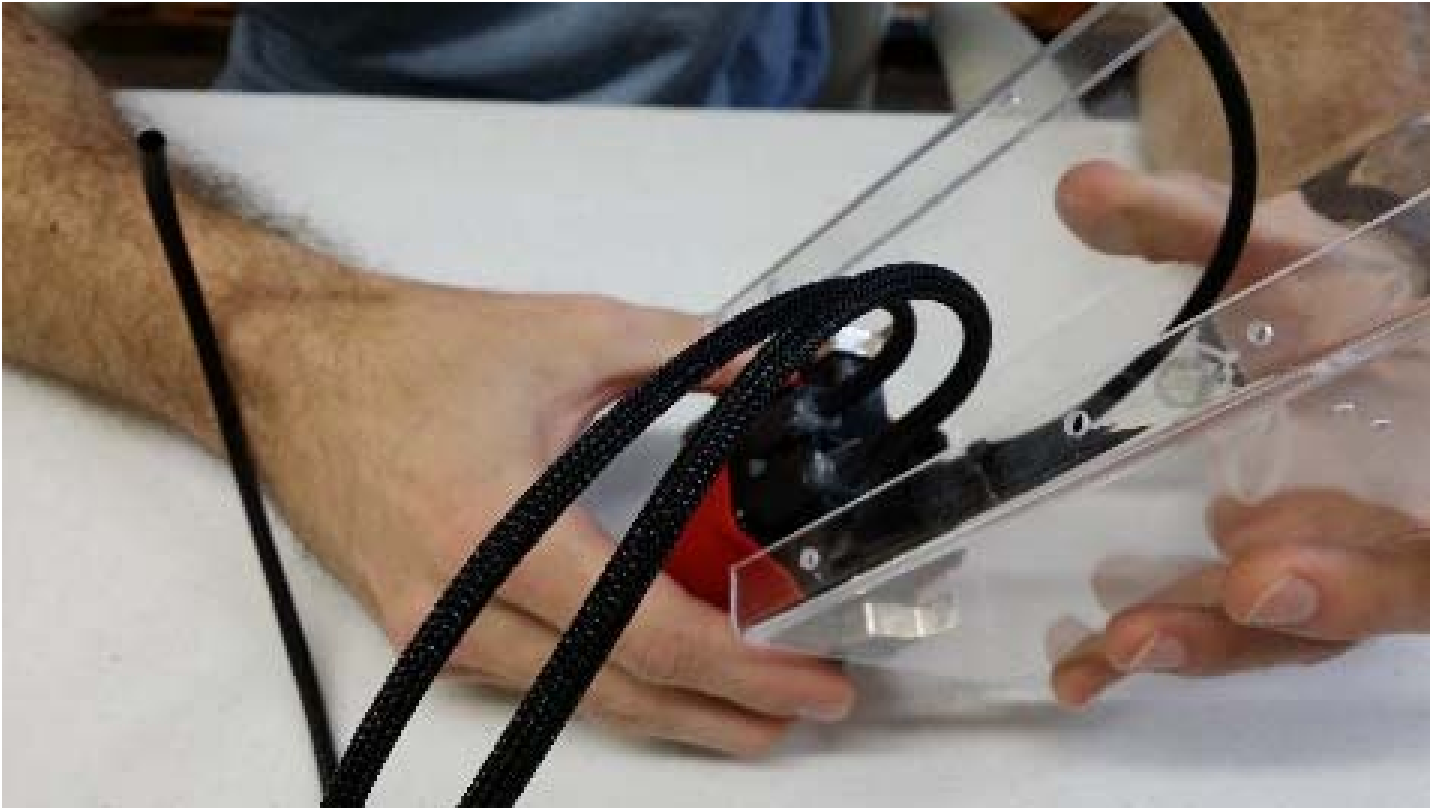
Slide HV Coil into position
