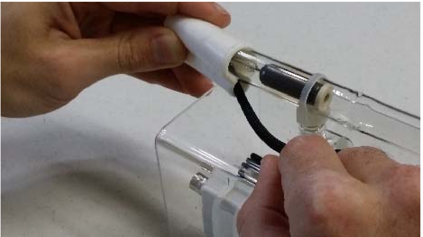
Holding wire in place, replace End Cap over tube and electrode
