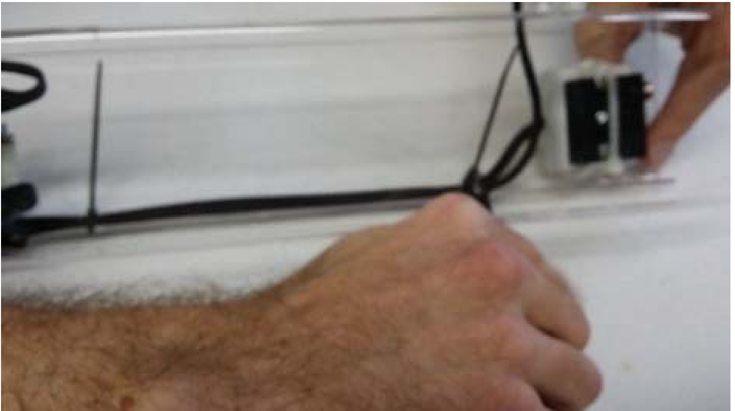
Route cables as shown and Tie-Wrap in place using holes on lower lip
