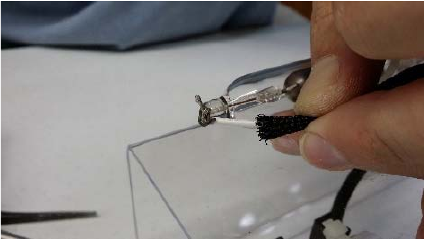
Carefully retract mesh sleeve to expose stripped Electrode Wire.
