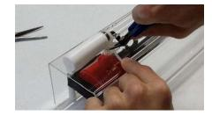
Clip off excess Tie-Wrap from Tube Mount
