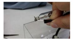
Carefully retract mesh sleeve to expose stripped Electrode Wire.
