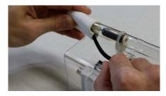
Holding wire in place, replace End Cap over tube and electrode
