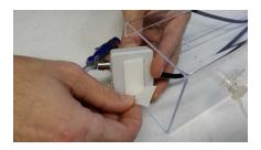
Mount Electronic Driver Module aligning between holes as shown
