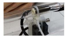
Position and Center tube on assembly. Snug up the incorporated Tie-Wrap to firmly hold tube in place
