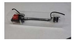
Route Tube electrodes wires through top of case as shown
