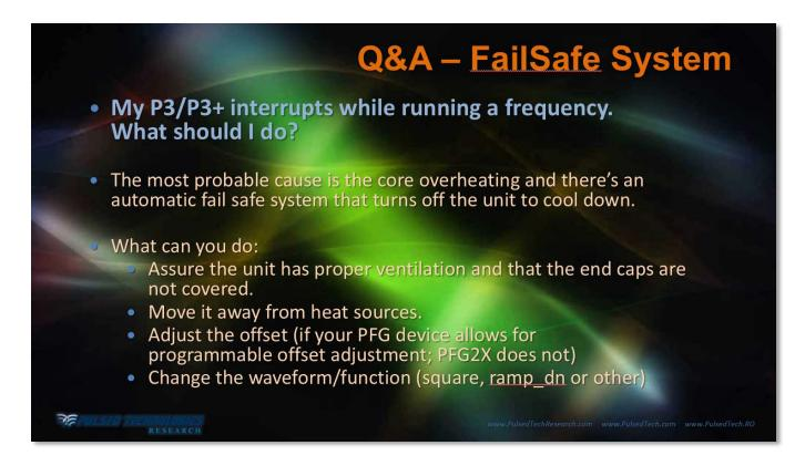
Pulsed Technologies P3, P3+, and P3pro plasma instruments all incorporate "failsafe" circuitry into their design. This helps protect circuitry and critical drive components from damage when "pushed" beyond thermal ranges. The system temporarily shuts down the drive circuitry until the issue is corrected or adjusted. While in this protection state, a specific LED indicator is illuminated. Reset typically happens automatically.
