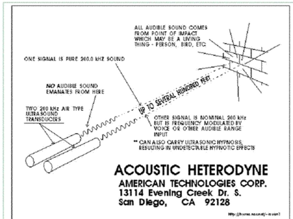
**Usage:** The [Audio Spotlight](#) can be used in two major ways: As directed audio, sound is directed at a specific listener or area, to provide a private or area specific listening space. As projected audio, sound is projected against a distant object, creating an audio image. This audio image is literally a projected loudspeaker - sound appears to come directly from the projection, just like light.
