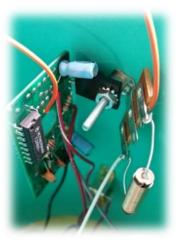
What was found consisted only of one IC (street value appx 52 cents retail), a power regulator (street value appx 75 cents) with the other support components typically a few cents or slightly more. The most expensive component appears to be the wall power supply or possibly the white PVC sewer end caps used to seal the unit.
