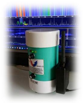
Total power draw was measured at 20ma which is about what you would expect the two flashing LEDs to use leaving practically nothing left to energize the touted coil (what appears to be a simple 3/4" RF choke). We WERE able to get readings by placing our sensors inside the unit directly on the emitting component, but even then at only very weak levels at a single frequency with pathetic waveform.
